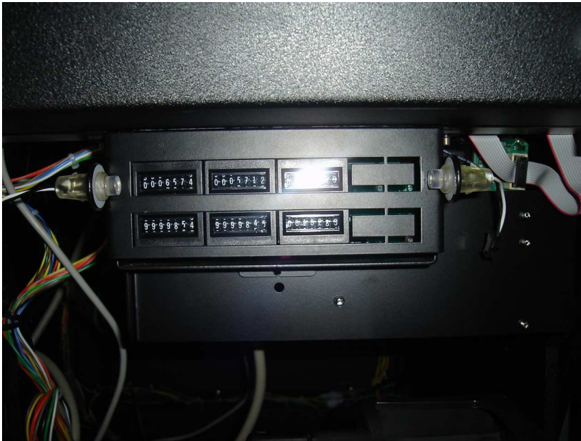
Figure 13: Hardware Meters Position in Machine
